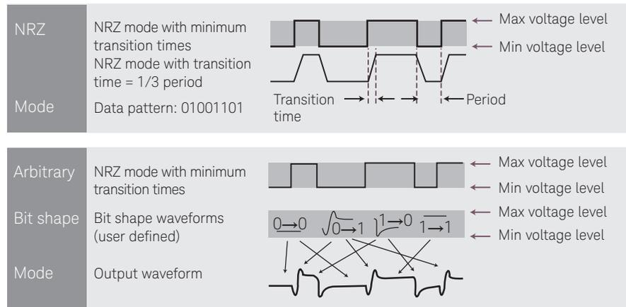
The 81150A and the 81160A pattern generators let you define the transitions from one bit to the other so that the previous bit influences the current bit. The user can set up own defined arbitrary bit shapes.
