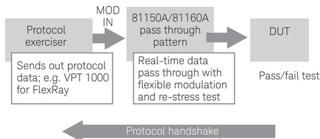
The pass-through pattern functionality takes the protocol data via Mod In and adds any kind of stress (shape and timing changes).
